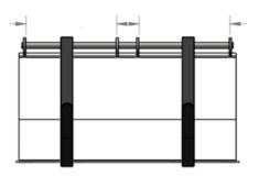
Complete welding the **Mounting Brackets to** the top of the Bucket:
